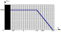
board (thermal resistance). The rated dissipation applies only if the permitted film temperature is not exceeded. These resistors do not feature a limited lifetime when operated within the permissible limits. However, resistance value drift increasing over operating time may result in exceeding a limit acceptable to the specific application, thereby establishing a functional lifetime.
